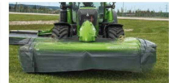
The +/- 5° swing means that the Fendt Cutter FPV can be adjusted to the ground, and that no stalk is left behind.
