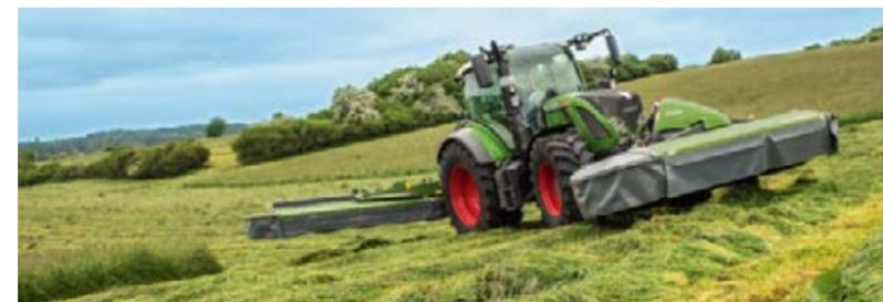
The generous ground clearance enables quick and safe turning on headlands, and the compensating cylinder on the outrigger keeps the mower stable on headlands.
